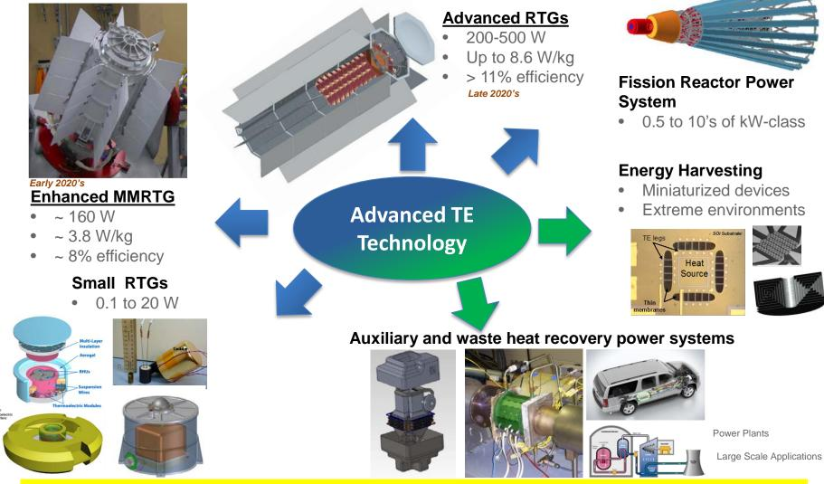
Advanced high temperature TE technology being developed for space power systems could also be applied to terrestrial Waste Heat Recovery and auxiliary power systems
