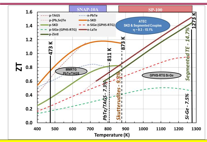
> 11% efficiency projected for ARTG based on 1273 K/523 K operating temperature differential (GPHS-RTG: 6.5%)
