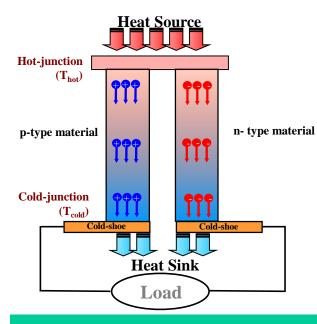
Thermoelectric effects are defined by a coupling between the electrical and thermal currents induced by an electric field and a temperature gradient
